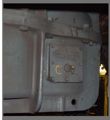
A Pitot tube provides the optimal method for sampling a gearbox.
